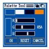
This program can change Workbench colour scheme. The colour scheme only lasts until the next reboot so you can save the changes only temporarily apply them to the workbench screen.
