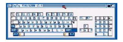
Displays the current keyboard characters using the current keymap. Pressing the CTRL, SHIFT or ALT keys will display the alternative keys when those keys are used. To change keymaps you must use the Setmap command and select a different mapping.
