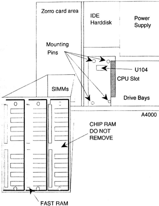
The SIMMs are located on the lower left of the motherboard. You will have to remove any expansion cards to see the SIMMs.
