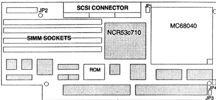
3. Set the chip down on the socket. When you have determined that all of the pins are resting in their socket holes, press the chip firmly down in the socket.
